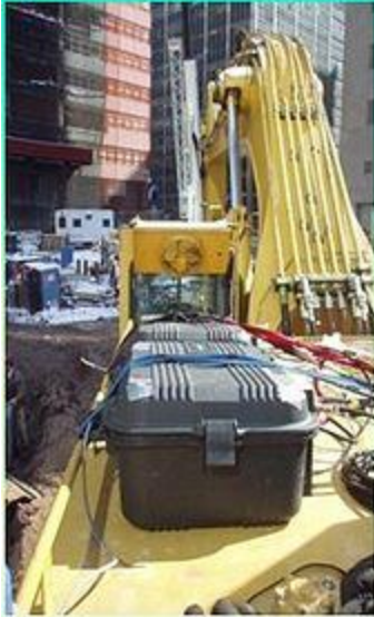
A CATI PEMS testing in the field at the World Trade Center in 2002
