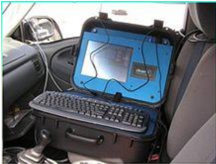
A PEMS being used to test a gasoline vehicle - 2002
