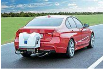
1065 PEMS manufactured by AVL - attached on a passenger car
