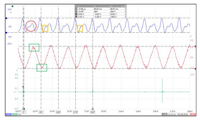
RPM = 30000 \* Nstrokes)/ (cycle time) = 120000 / 80.97 = 1482 by aligning the spark events.
