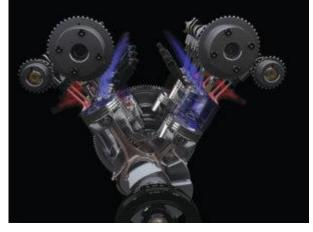
intake valve is dropping into a combustion chamber with combustion byproducts or unburned fuel, the valve might be exposed to the precursors that cause carbon build-up. Some have blamed the positive crankcase ventilation (PCV) systems for leaving an oily film on the intake valve that is then baked into carbon. Some blame the valve overlap during the intake stroke that eliminates the need for an EGR valve.
