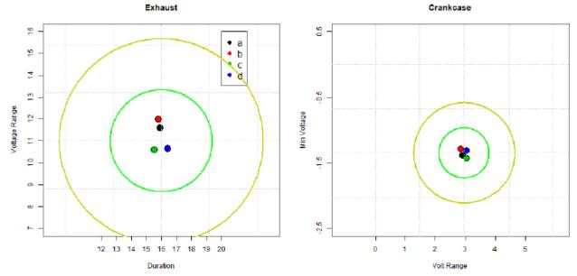
Each cylinder in firing order sequence, as shown in the legend, is plotted to show the (dis)similarity of the behavior in each cylinder. The voltage is in direct proportion to the pressure sensed and the duration is in milliseconds. Ideally, the points would be right on top of each other; if they are in the interior green circles, the cylinders are quite good.
