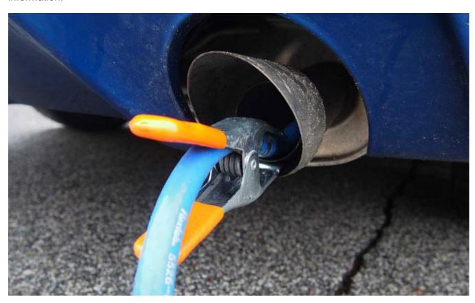
These instruments attach to something known as a PicoScope, which interacts with Engine Polygraph software running on a computer, helping turn raw data into readable graphs and ultimately an overall rating for the powerplant being evaluated.
